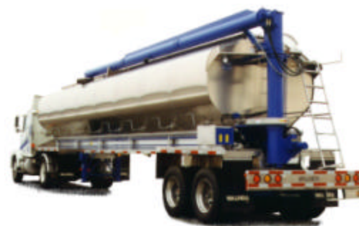
Walinga’s most popular product line, pictured is a “demo” aluminum feed hopper trailer with integrated boom auger discharge system.
