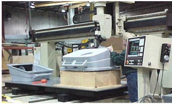
Post mold parts trimming on Five Axis CNC Router
